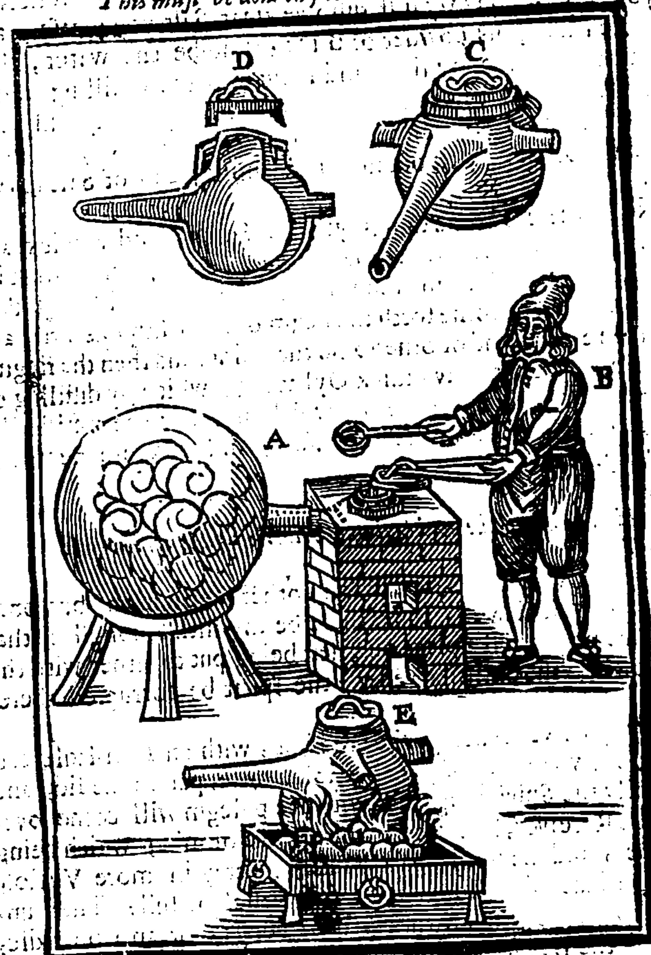
A Signifies the Furnace with its Iron, or earthen distilling vessel, walled in, to which a very large Receiver is joyned. B, the Distiller, who with his left hand inserteth of the cover, and with his right casteth in his prepared matter with an Iron-ladle. C, the form of the distilling vessel. D, the same, as it appeareth inward. E, the form of the vessel walled in, but standing on the coals for other uses.
