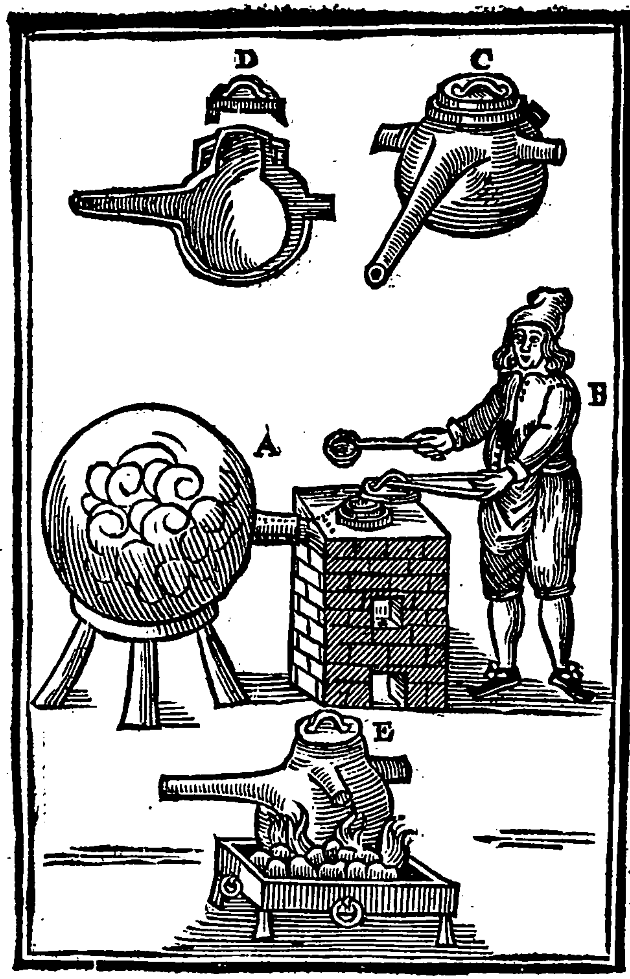
A. The furnace together with the iron distilling-vessel fastened into it, whereunto a receiver is applied. B. The distiller with his left hand taking off the lid, and with his right casting in his prepared matter. C. The external form of the distilling vessel. D. The internal form of the vessel. E. Another distilling vessel, which is not fastened to a furnace, but only standeth upon coals.
